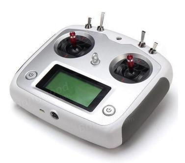
Our simulator uses the Flysky FS-16S controller which is very similar to the controllers used with the DJI drones. The controller is connected to the computer running the simulator by a USB cable. To turn on the controller, all top switches have to be in their upmost position and both power buttons have to be pressed simultaneously. Similarly, to turn the controller off, both power buttons have to be pressed.
